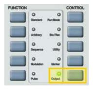
**13.** Define the channels in the **Output** section as being ON or OFF, modifying the settings using the dial or the cursor keys.
